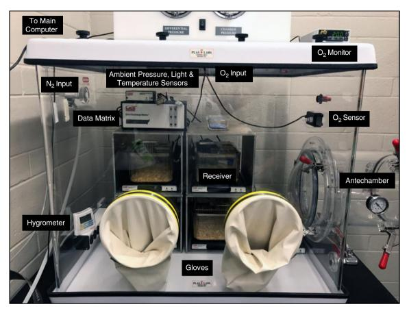
**Figure 1. Experimental set-up**Hypoxia chamber and telemetry unit set-up. [Colour figure can be viewed at wileyonlinelibrary.com]
